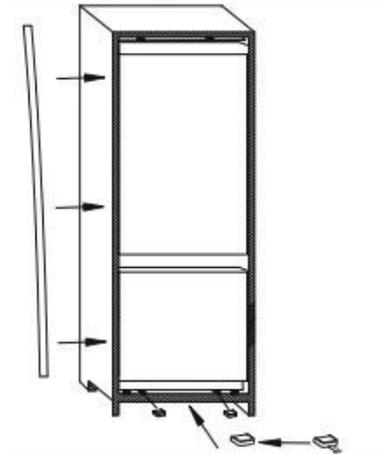
Fit the seal to the appliance, cut off the excessive part if necessary. Fit the bottom parts with plastic covers
