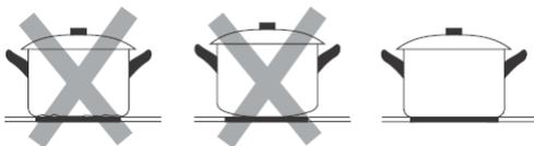
Make sure that the base of your pan is smooth, sits flat against the glass, and is the same size as the cooking zone. Use pans whose diameter is as large as the graphic of the zone selected. Using a pot a slightly wider energy will be used at its maximum efficiency. If you use smaller pot efficiency could be less than expected. Always center your pan on the cooking zone.
