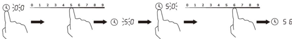
3. Cancel the time by touching the Timer button, the left symbol of time indicator will start flashing, touch the "0" on the slider within 5s. Then touch the Timer button again within 5s, the left symbol will stop flashing and the right symbol of time indicator will start flashing, touch the "0" on the slider within 5s.
