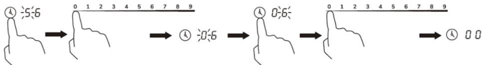
4. When the time is set, it will begin to count down immediately. The display will show the remaining time and the timer indicator will flash for 5 seconds.
