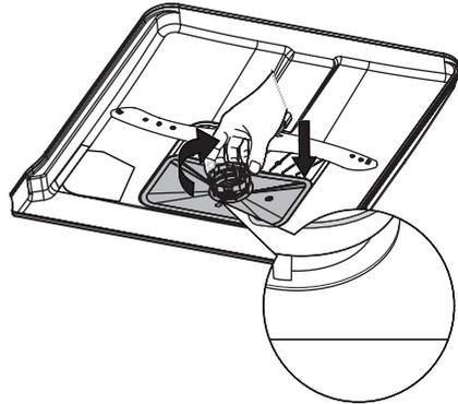
Reassemble the filters in the reverse order of the disassembly, replace the filter insert, and rotate clockwise to the close arrow
