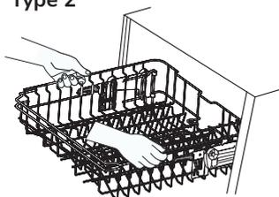
To raise the upper basket, just lift the upper basket at the center of each side until the basket locks into place in the upper position.
