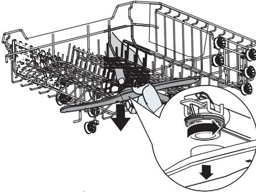
To remove the upper spray arm, hold the nut in the center still and rotate the spray arm counterclockwise to remove it
