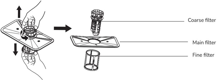
The fine filter can be pulled off the bottom of the filter assembly. The coarse filter can be detached from the main filter by gently squeezing the tabs at the top and pulling it away
