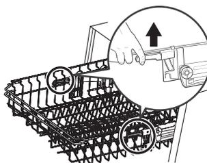
To lower the upper basket, lift the adjust handles on each side to release the basket and lower it to the lower position
